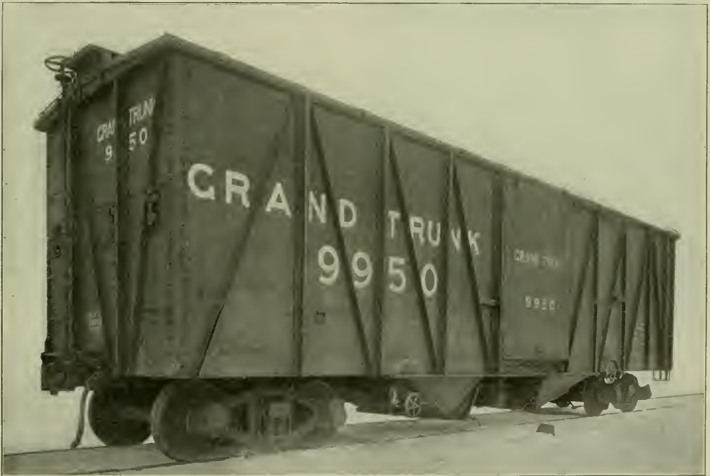
Steel Frame Box Car Equipped with a Hopper Bottom.
